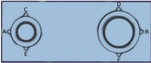
Fig. 4. Reference points from A to F. For accurate margin measurement, the reference points were used for sectioning the reconstructed CT data in the desired planes.
