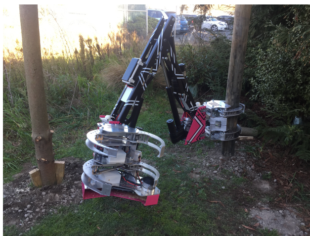
Figure 3. Tree to tree robot (image taken by SCION NZ Forest Research Institute, used with permission from Richard Parker).
