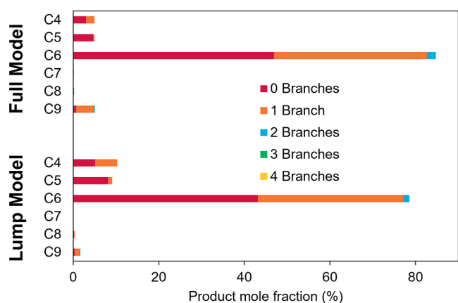
Figure 13. Product mole fractions for full and lump model simulations. Fractions were calculated with respect to the entire product distribution (C4–C9). Conversion for both simulations was about 1%.
