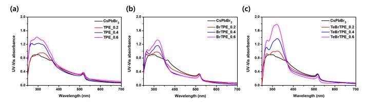
**Figure 3.** Absorption spectra of perovskite films with various molar ratios of TPE derivatives: (a) CsPbBr<sub>3</sub> perovskite films with TPE/CsPbBr<sub>3</sub> molar ratios of 0.2, 0.4, and 0.6; (b) CsPbBr<sub>3</sub> perovskite films with BrTPE/CsPbBr<sub>3</sub> molar ratios of 0.2, 0.4, and 0.6; and (c) CsPbBr<sub>3</sub> perovskite films with TeBrTPE/CsPbBr<sub>3</sub> molar ratios of 0.2, 0.4, and 0.6.
