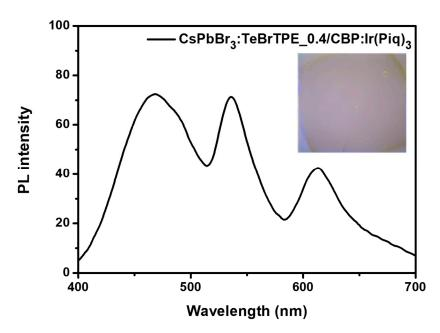
**Figure 6.** White-light PL spectrum of a vacuum-deposited film of a red emitter on a CsPbBr<sub>3</sub> film with a BrTPE/CsPbBr<sub>3</sub> molar ratio of 0.4 (excitation wavelength: 300 nm), inset: optical photograph under irradiation of 365 nm.
