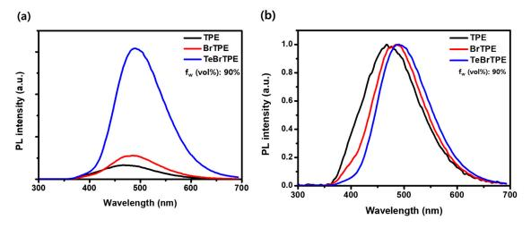
**Figure 2.** (a) Fluorescence spectra of TPE derivatives in THF (10 vol%) and water (90 vol%) solvents; (b) Normalized fluorescence spectra of TPE derivatives in THF (10 vol%) and water (90 vol%) solvents.
