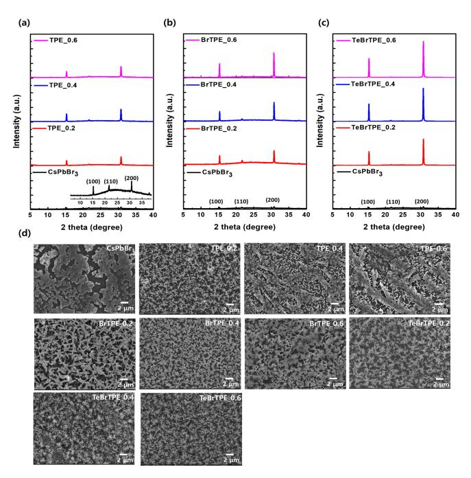
**Figure 5.** Crystal structures and morphologies of CsPbBr<sub>3</sub> thin films with 0.2, 0.4, and 0.6 mol of TPE, BrTPE, and TeBrTPE per mole of CsPbBr<sub>3</sub>. (**a–c**) X-ray diffraction (XRD) patterns and (**d**) top-view scanning electron microscopy (SEM) images  $(25,000\times$ , scale bar: 2  $\mu$ m).
