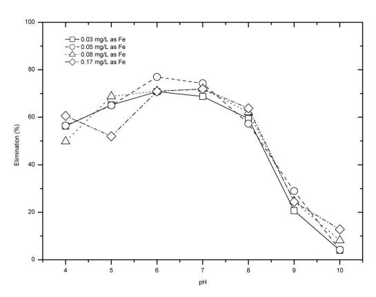
Figure 7. CIP removal of samples with various final pH for various ferrate doses.  $\verb|doi:10.1371/journal.pone.0055729.g007|$
