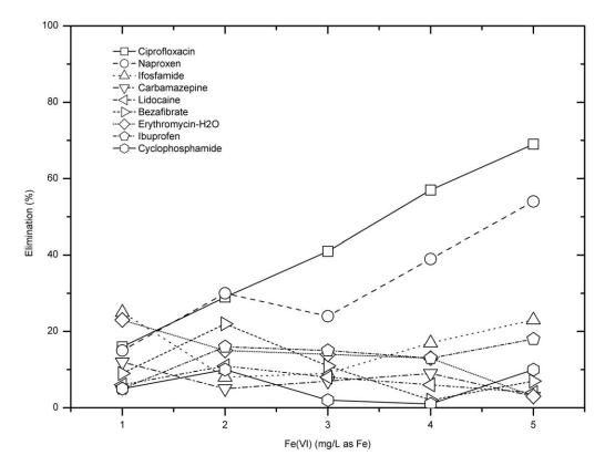
Figure 8. Pharmaceuticals removal by ferrate at pH 6. doi:10.1371/journal.pone.0055729.q008
