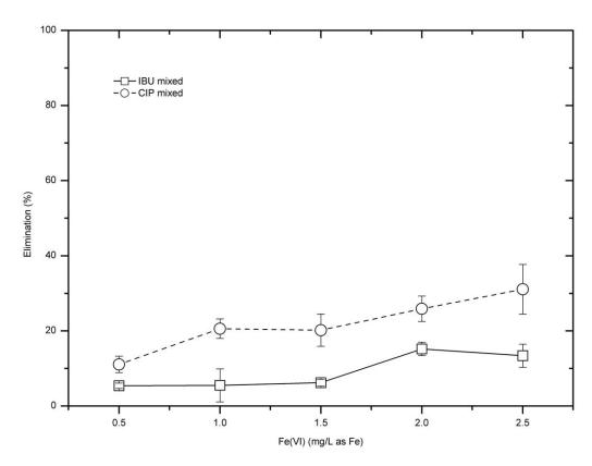
Figure 4. Experimental results of 10  $\mu$ g/L IBU and CIP mixed model test solutions (pH = 7.05  $\pm$  0.25). doi:10.1371/journal.pone.0055729.g004
