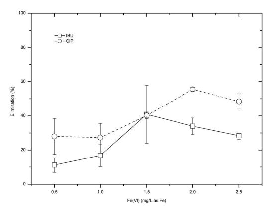
Figure 3. Treatment of 10  $\mu$ g/L IBU model water samples by ferrate (VI) (pH = 7.05  $\pm$  0.25). doi:10.1371/journal.pone.0055729.g003
