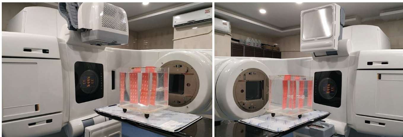
Figure 2. Arrangement of the water phantom with samples on the right and left side of the linear accelerator machine in order to receive bilateral radiation.
