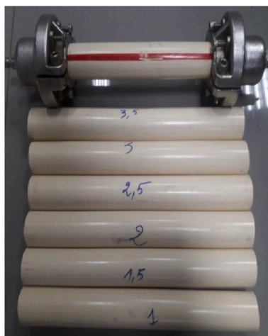
Fig. 1. Notched tubes for burst test.
