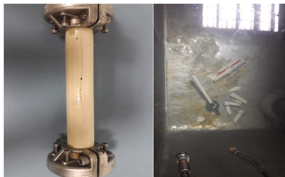
Fig. 3. Fracture shapes of CPVC specimens after bursting test.
