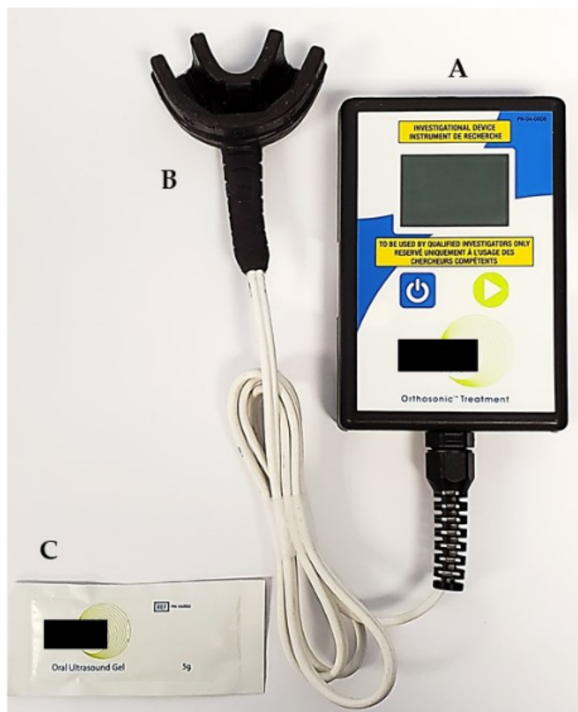
Figure 2. Low-intensity pulsed ultrasound (LIPUS) device used in the clinical trial including A: handheld electronics; B: mouthpiece containing LIPUS transducers; and, C: oral ultrasound gel.
