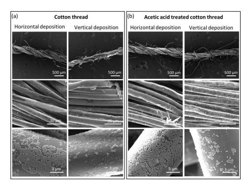
**Figure 2.** Representative SEM images for horizontal and vertical deposition of metal-organic framework (MOF) nanoparticles (NPs) onto pristine cotton thread (left, **a**) and cotton thread treated with acetic acid (right, **b**). From top to bottom, each column shows the increased magnification of the threads.
