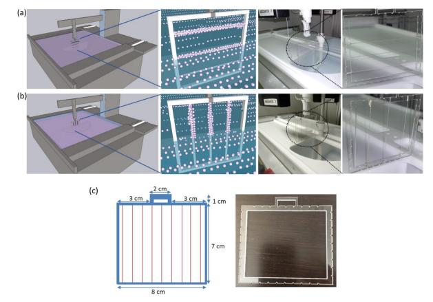
**Figure 1.** Schematic depiction and photograph of the setup used for Langmuir-Blodgett (LB) deposition in horizontal (**a**) and vertical (**b**) configurations of the fiber or threads. (**c**) Dimensions and picture of the holder showing vertical and horizontal grooves for fixing the fiber or threads.
