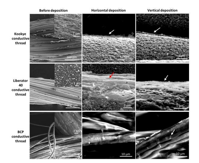
**Figure 4.** SEM images of the three conductive threads studied, as indicated, prior to deposition (**left**), after LB deposition of MOF NPs in horizontal (**middle**) and vertical (**right**) configurations. The red and white arrows highlight the MOF NPs deposits.
