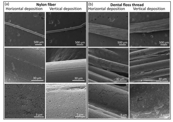
**Figure 3.** Representative SEM images for horizontal and vertical deposition of MOF NPs onto nylon fiber (left, **a**) and dental floss thread (right, **b**). From top to bottom, each column shows increased magnification.
