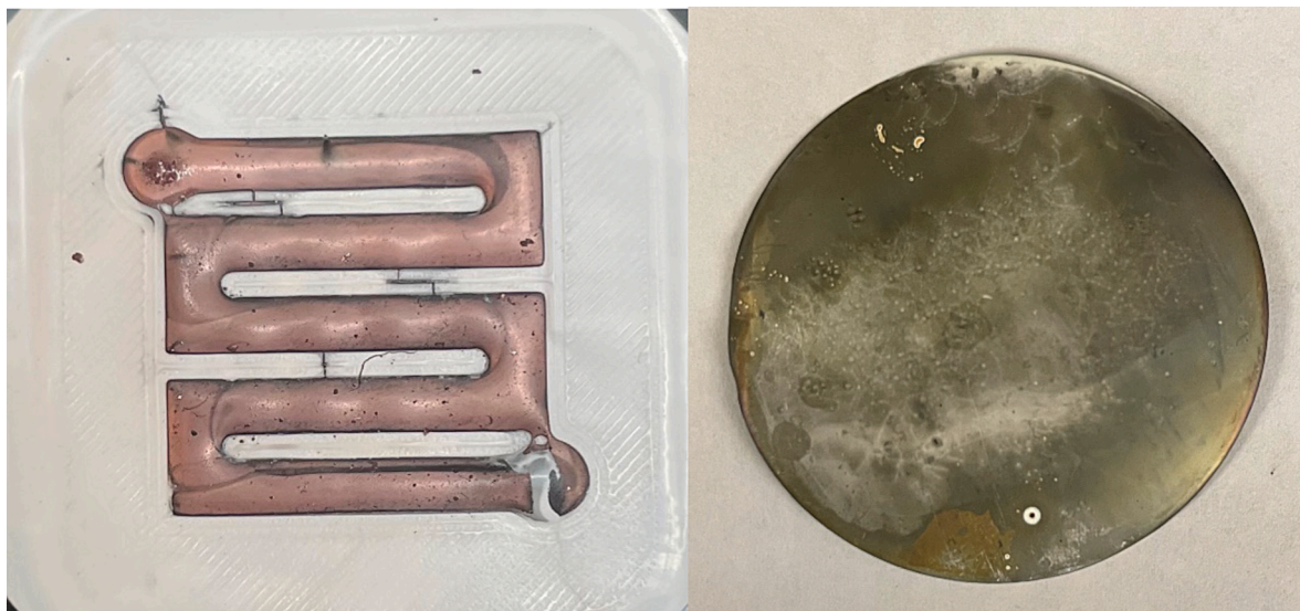
Fig. 8. Electroless deposition of copper plating solution using the serpentine pattern on the 3D printed flow cell is shown on the left. On the right is electroless deposition of copper plating solution onto a PES membrane using typical submersion techniques.
