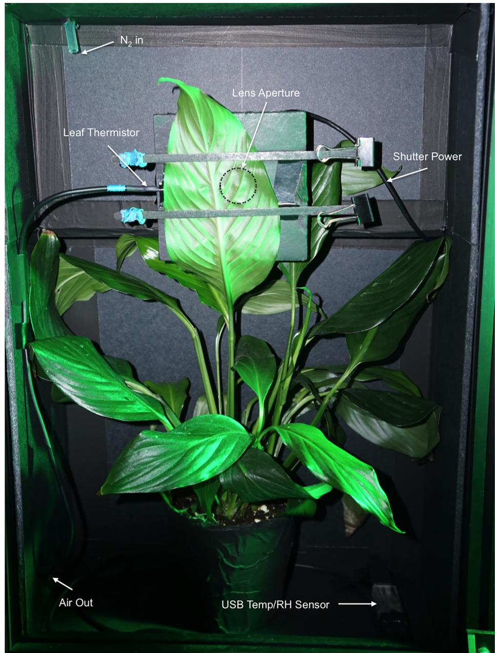
**Fig 18. Plant test enclosure.** *Spathiphyllum* in plant enclosure (S). Shown with single filter lens assembly and front panel removed.
