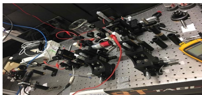
Figure 9. The schematic diagram of the laser setup for the characterization process of nano-antennas.
