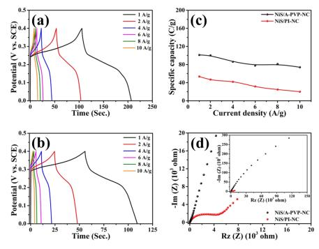
**Figure 6.** Galvanostatic charge–discharge profiles of NiS/A-PVP-NC (**a**) and NiS/PI-NC (**b**), their specific capacities as functions of the current densities (**c**), and electrochemical impedance spectra (**d**).
