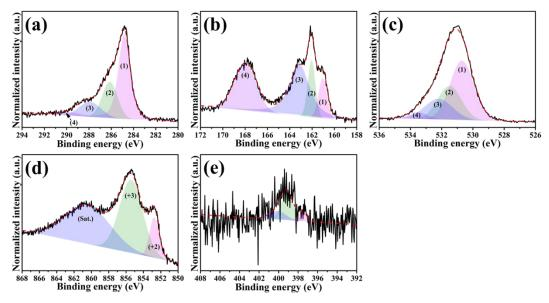
**Figure 3.** High-resolution XPS spectra of the NiS/A-PVP-NC: (a) C 1s ((1) for C=C bond, (2) for C=O bond, (3) for C=O bond, and (4) for O=C=O bond), (b) S 2p ((1)–(3) assigned to  $S^{2-}$  within the NiS, and (4) obtained from sulfate ions), (c) O 1s ((1) and (3) associated with the Ni<sup>3+</sup>OOH and Ni<sup>2+</sup>SO<sub>4</sub>, (2) for O=C=O bond, and (4) for C=O bond), (d) Ni 2p and (e) N 1s.
