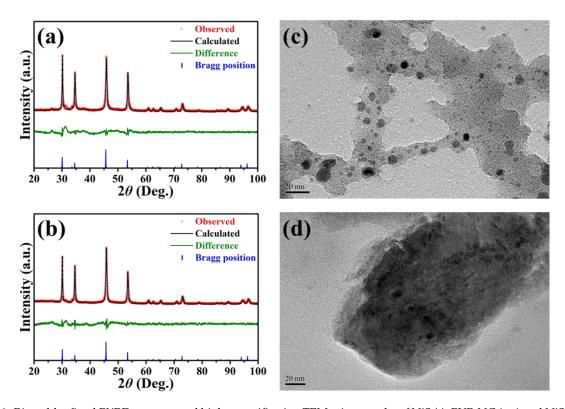
**Figure 2.** Rietveld refined PXRD patterns and high-magnification TEM micrographs of NiS/A-PVP-NC (a,c) and NiS/PI-NC (b,d). Scale bars of (c,d) are 20 nm.
