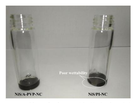
Figure 4. Wettability test of NiS/A-PVP-NC (left side) and NiS/PI-NC (right side).
