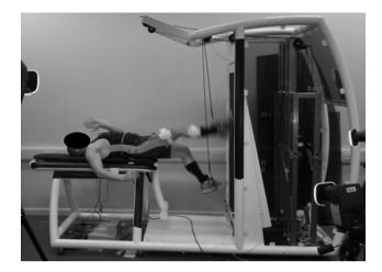
Fig. 1. The VertiRun (Sheffield, UK) being used in the supine posture.
