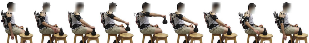
Figure 6. The participant is wearing the active exoskeleton and sensors while doing a weight-lifting task in the sagittal plane.
