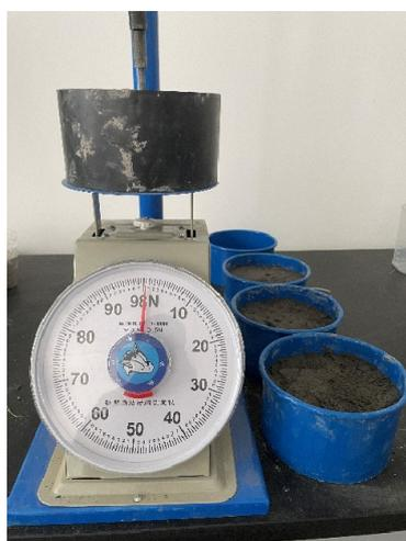
**Figure 4.** Setting time tester of mortar.
