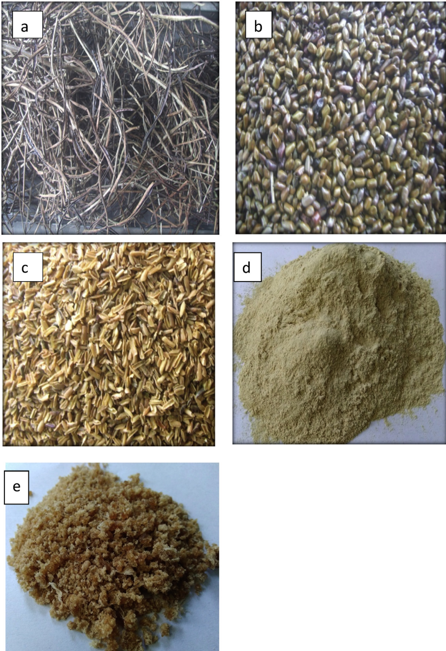
Fig. 1. Optical images of (a) legumes from Cassia tora plant (b) seeds of Cassia tora (c) endosperm of Cassia tora (d) Cassia tora gum (e) quaternized Cassia tora gum.
