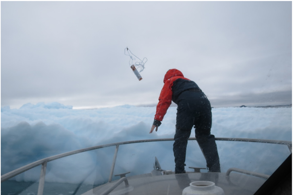
Fig. 2. An expendable ice tracker (EXITE) deployed by hand. The EXITE was simply thrown from a small boat onto a drifting iceberg.
