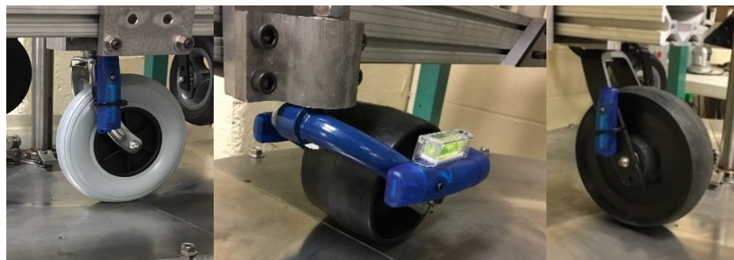
Fig 6. Accelerometers installed on test castors. The Hopehaven castor (left) is a 185mm solid tyre castor that mounts on a plastic castor wheel. The Whirlwind castor (middle) is a 127mm solid tyre castor mounted on the axle bearing similar to the Motivation castor (right) which is a heavy, 216mm solid castor.
