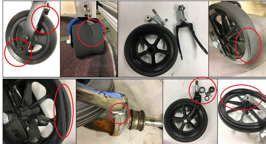
Fig 17. Model A–Delaminated tyre brushing against the fork (top-left), Model B–Tyre cracking (top-left-middle), Model C–Axle hub assembly fell apart (top-right-middle), Model D–Tyre Cracking (top-right), Model E–Tyre Cracking (bottom-left), Model F–Fork fracture (bottom-left-middle), Model G–Stem bearing fracture (bottom-right-middle) and Model H–Wheel Fracture (bottom-right).
