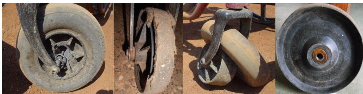
Fig 1. Castor axle bearing failure (left), tire cracking and worn-out (middle left), tire Roll-off (middle-right) and axle bearing corrosion (right).
