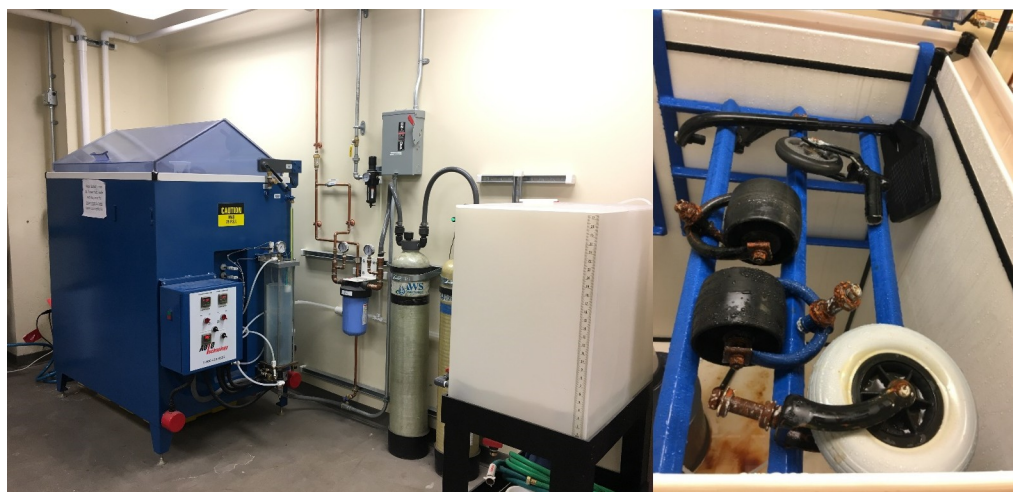
Fig 7. Salt fog chamber for corrosion testing (left) and corrosion testing of sample parts (right) [50].
