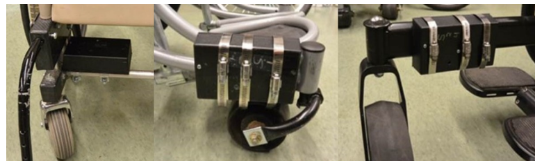
Fig 5. Accelerometers installed in a black box attached to the wheelchair frame.
