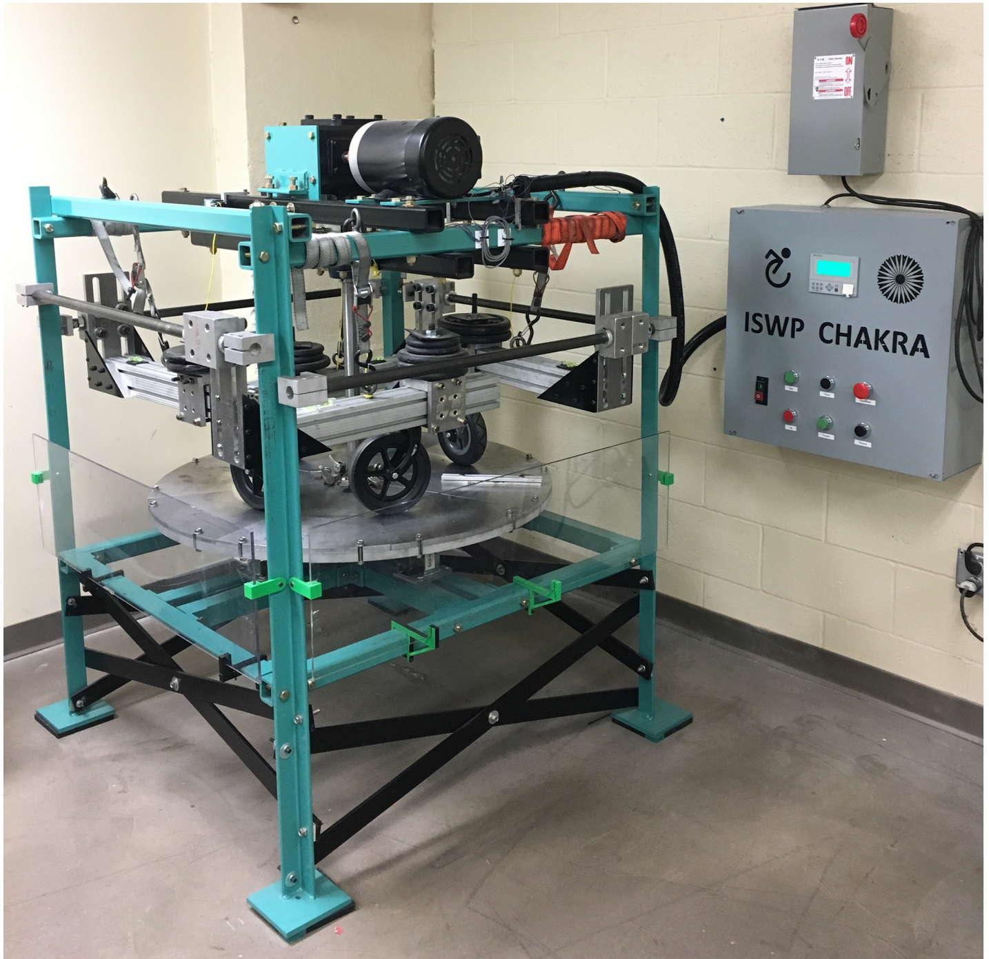
Fig 2. ISWP castor testing system.
