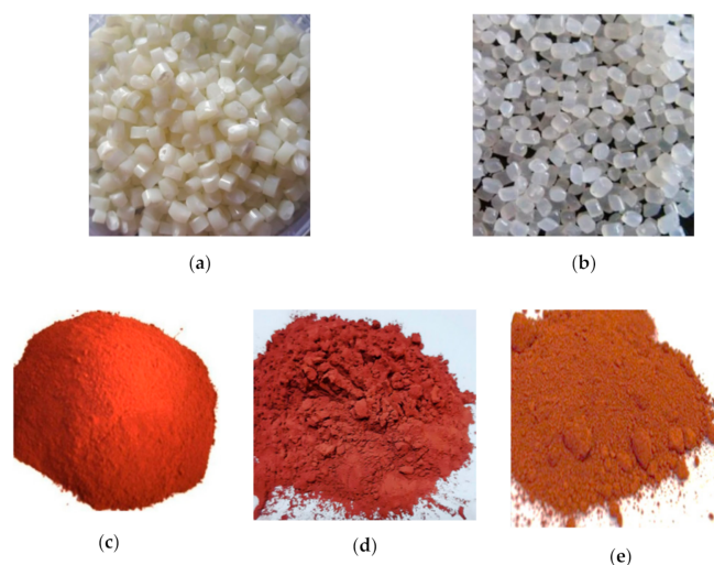
Figure 1. Images of: (a) ABS, (b) nylon 6, (c) 100 mesh copper powder, (d) 200 mesh copper powder, and (e) 400 mesh copper powder.
