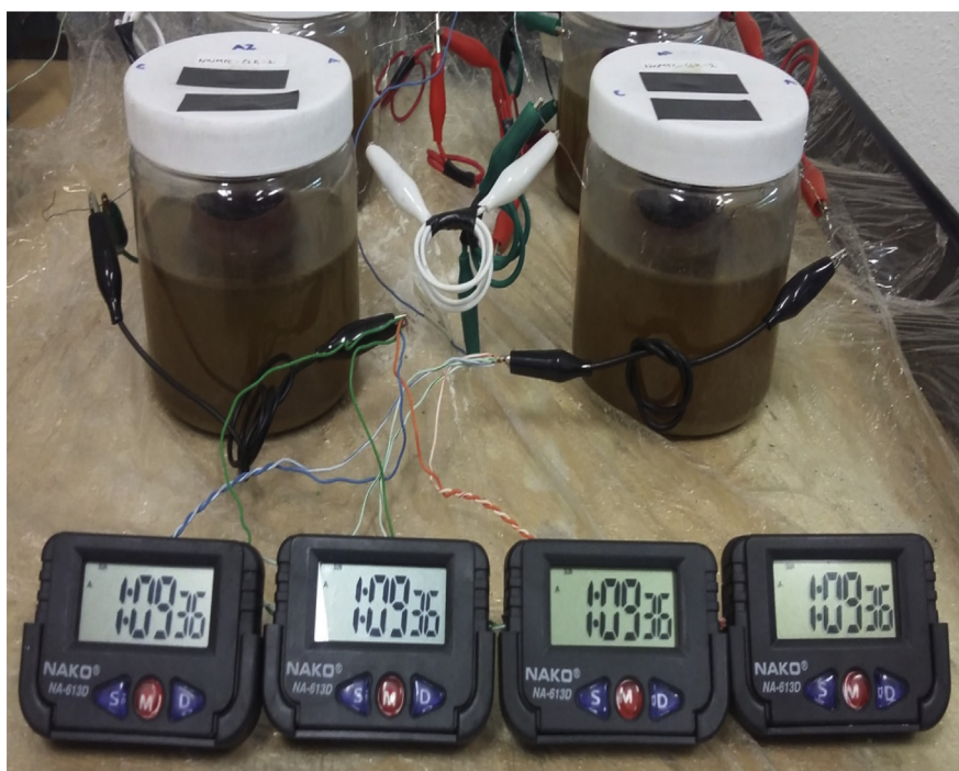
Fig. 5. Both-C-MFCs connected in series in order to power the digital clocks.
