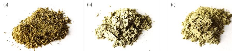
Figure 1. Optical image of (a) non-functionalized lavender filler, (b) lavender filler functionalized with kaolinite, and (c) lavender fillers functionalized with hydroxyapatite.
