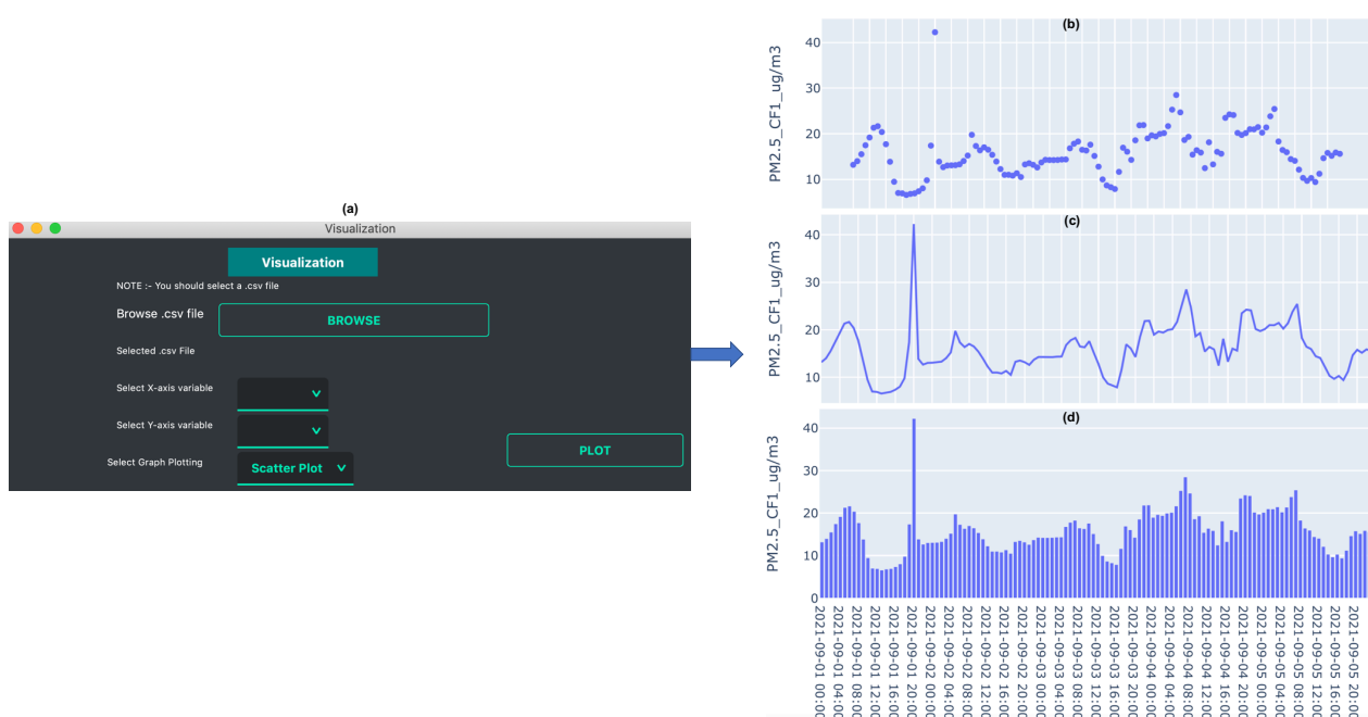
Figure 2. Data visualization example: (a) Snapshot of data visualization GUI, (b) scatter plot, (c) line plot, and (d) bar plot.
