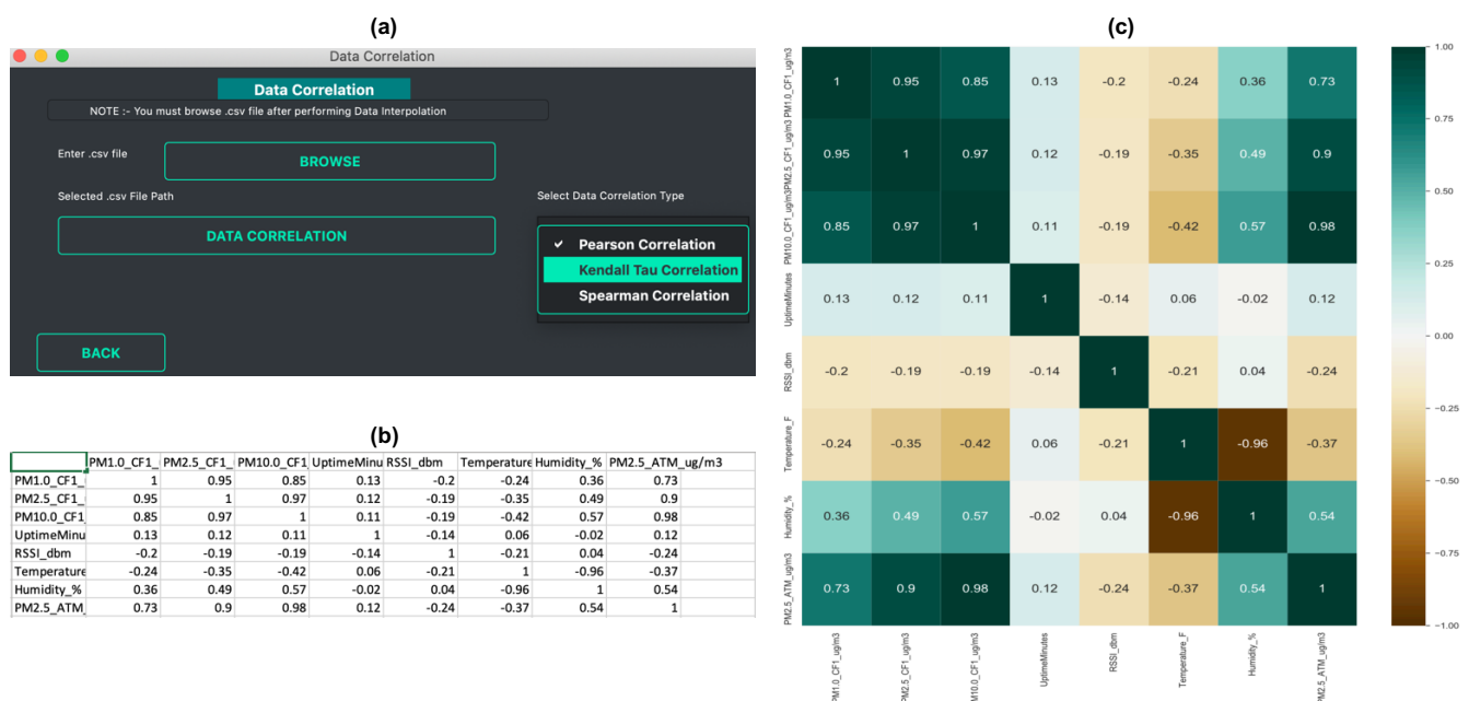
Figure 4. Data correlation example: (a) Snapshot of data correlation GUI, (b) output as a CSV file, and (c) correlation heatmap.
