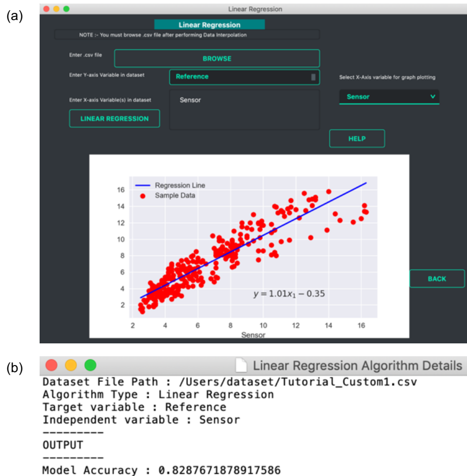
Figure 5. Linear regression example: (a) Snapshot of linear regression GUI with regression plot and (b) snapshot of the text file showing regression model details.
