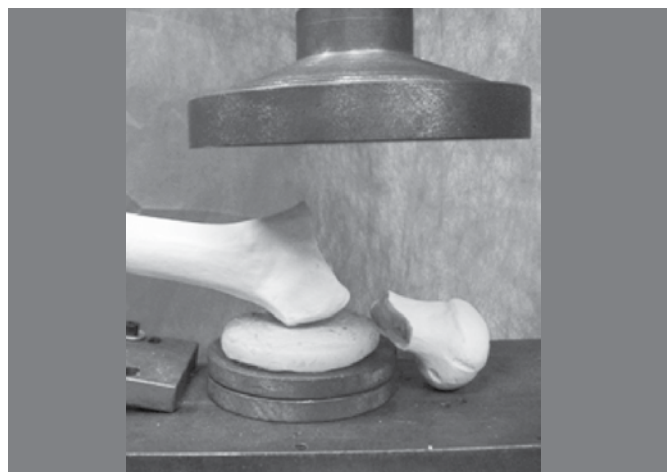
Figure 6. Sample of the DX group post-assay, showing the fracture of the femoral neck in the basicervical region.
