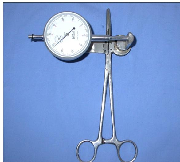
**Fig. 5.** Device used for measuring tension. A dynamometer was attached to haemostatic forceps.
