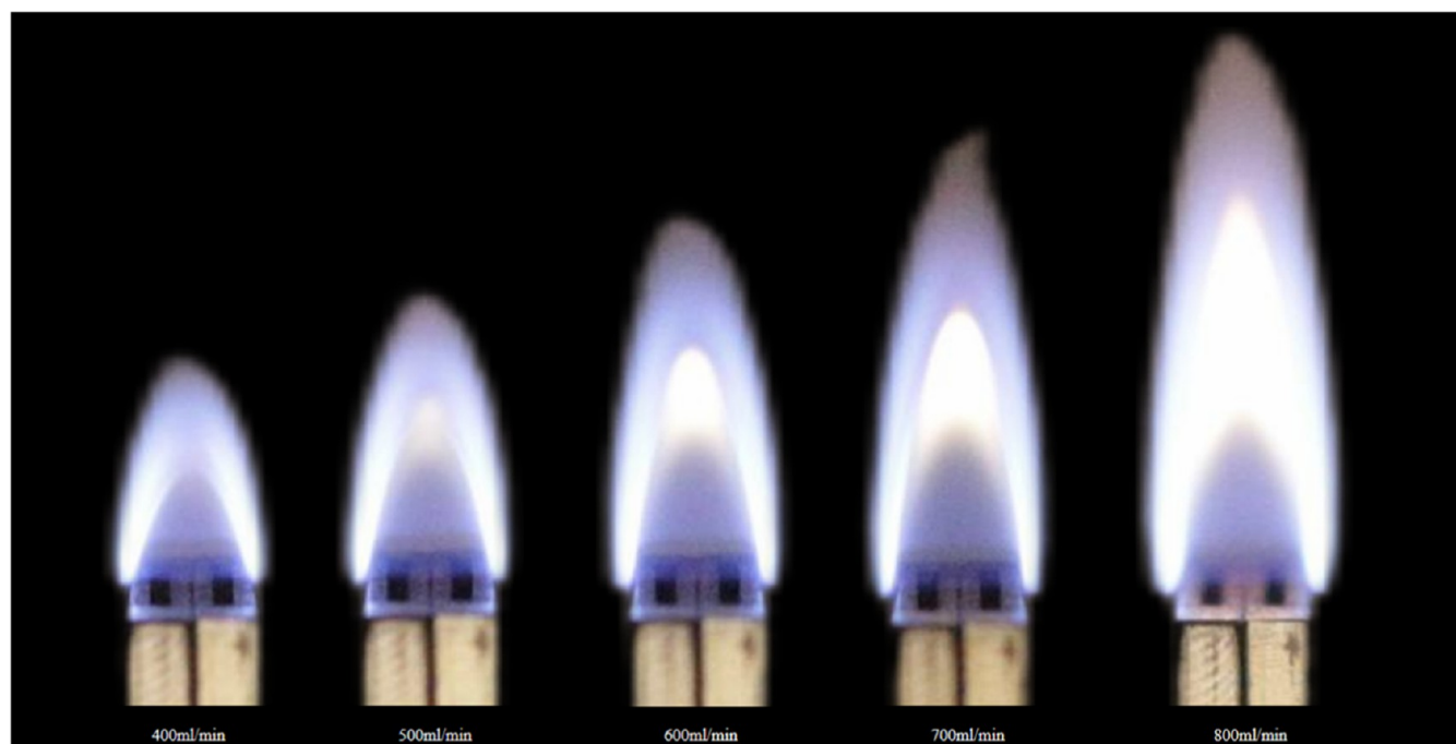
Figure 13. Flame appearance at 0 mm pitch for 50%CH 4 –50%NH 3 fuel at different flow rates (from left to right total flow rate in the order of 400, 500, 600, 700, 800 mL/min).
