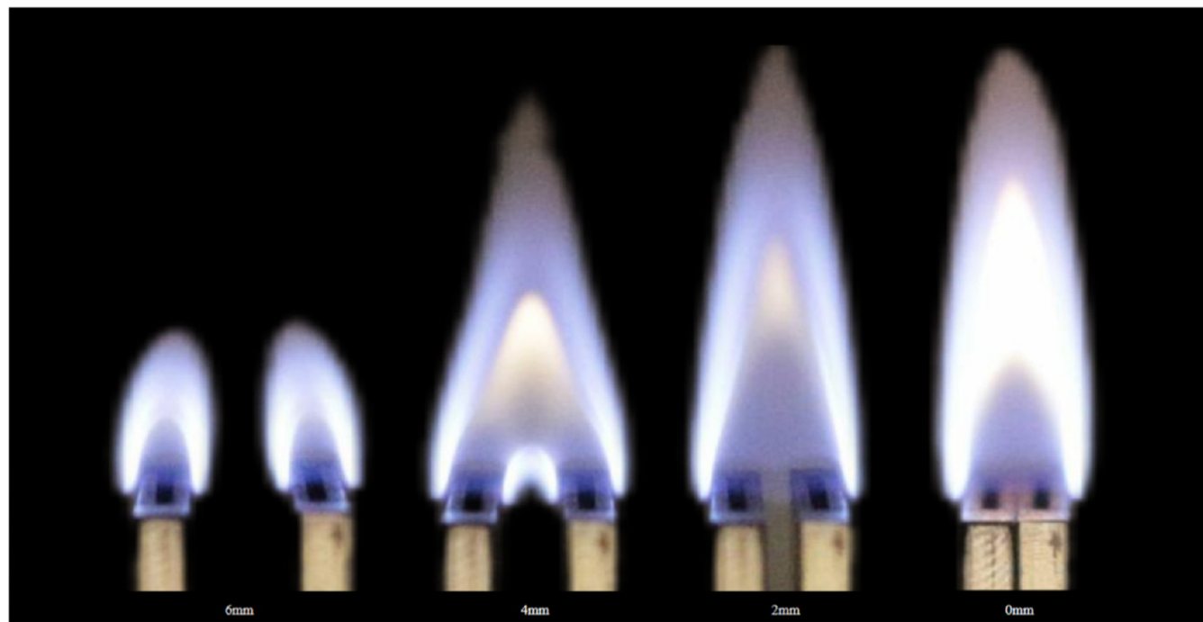
Figure 22. Flame appearance for a total flow rate of 800 mL/min and a blending ratio of 50%CH 4 –50%NH 3 fuel burning at different pitches (from left to right burner pitch is 6, 4, 2, 0 mm).
