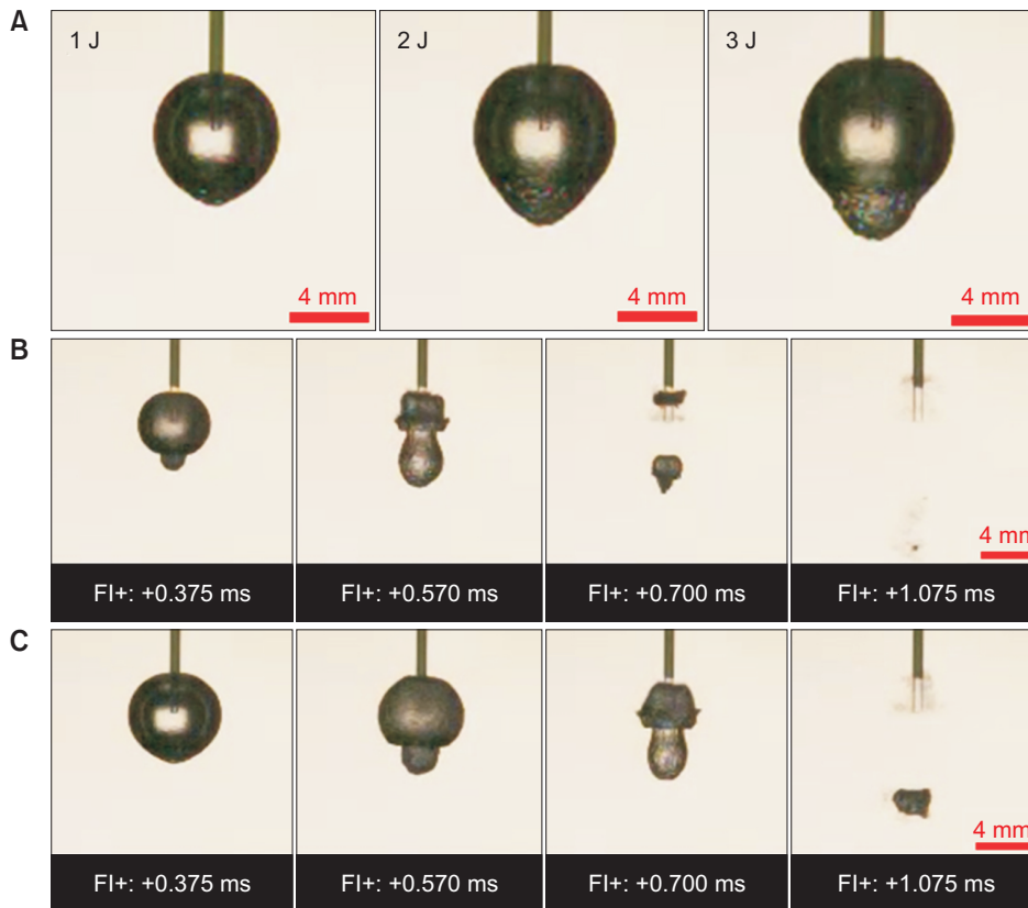
Fig. 6. (A) Differences in laser-induced cavitation bubble size according to a laser setting of 200,000 FPS. Formation of cavitation bubbles using MOSES technology in the contact mode (B) and distance mode (C). FI, from first image.
