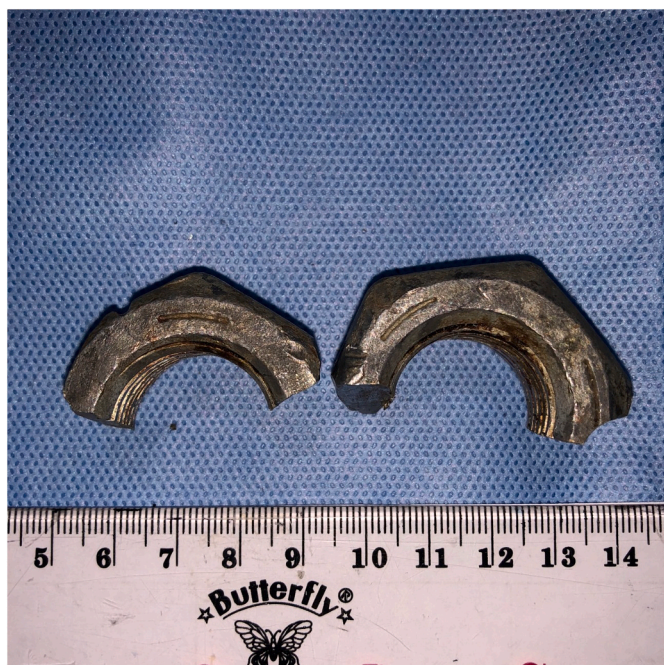
Fig. 1. Bolt ring after cut into two pieces.
