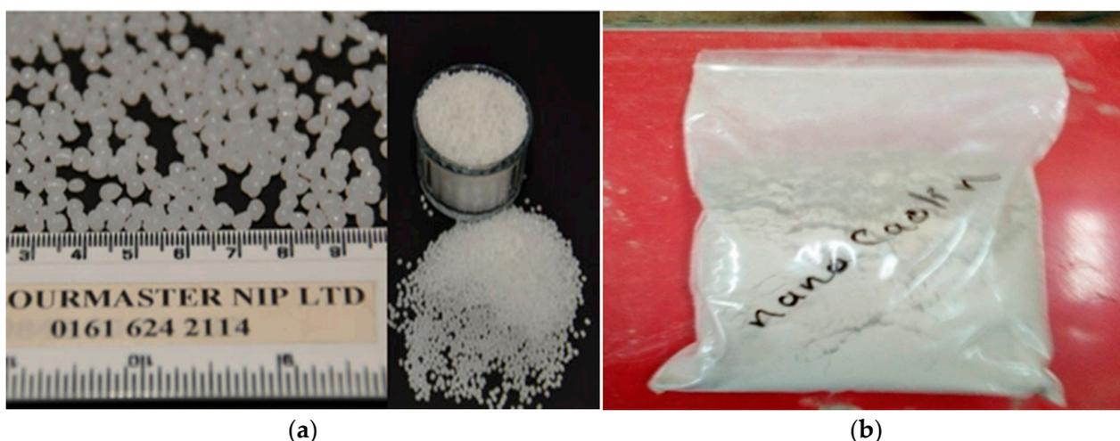
**Figure 1.** Utilized additives; (a) high-density polyethylene (HDPE) resin; (b) nanoclay (NC) powder.
