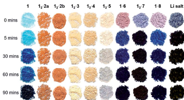
Fig. 9 The cofomer 1 and cocrystals 1_2 \cdot 2 , 1_2 \cdot 3 and 1_2 \cdot 4 , and salts 1_2 \cdot 5 , 1 \cdot 6 , 1_2 \cdot 7 , 1 \cdot 8 and the lithium salt (Li salt) before and after UV irradiation at 254 nm for different durations. The 1_2 \cdot 2a sample was irradiated with UV light at 365 nm while 254 nm radiation was used for the 1_2 \cdot 2b sample. The initial colour changes to UV radiation show that only 1 and the salt samples visibly change colour with prolonged irradiation, with 1_2 \cdot 7 being the most radiation sensitive to the naked eye and experimentally.
