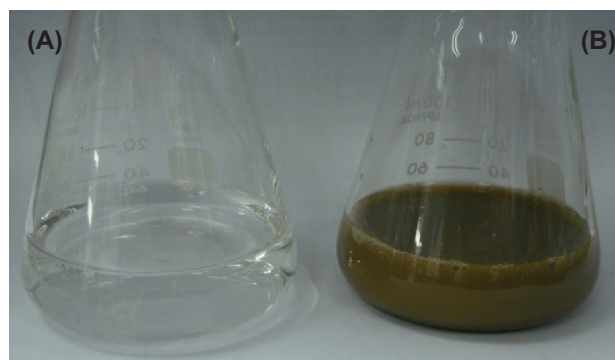
Figure 1 Aqueous solution of 10^{-3} \text{ M AgNO}_3 with pu-erh tea leaves extract (A) before adding the tea extract and (B) after addition of tea extract at 5 minutes.
