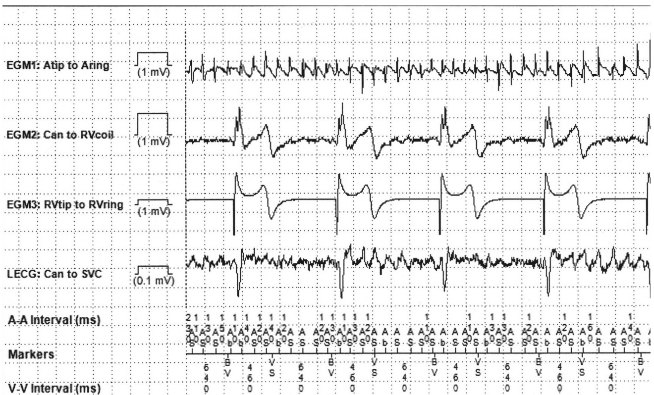
Figure 2 Medtronic electrograms showing high-amplitude postpacing T wave. T-wave oversensing persisted despite adjustments to sensitivity up to 1.2 mV, increase in postpacing blanking period to 400 ms, and changing lead sensing configuration from dedicated bipolar to integrated bipolar.
