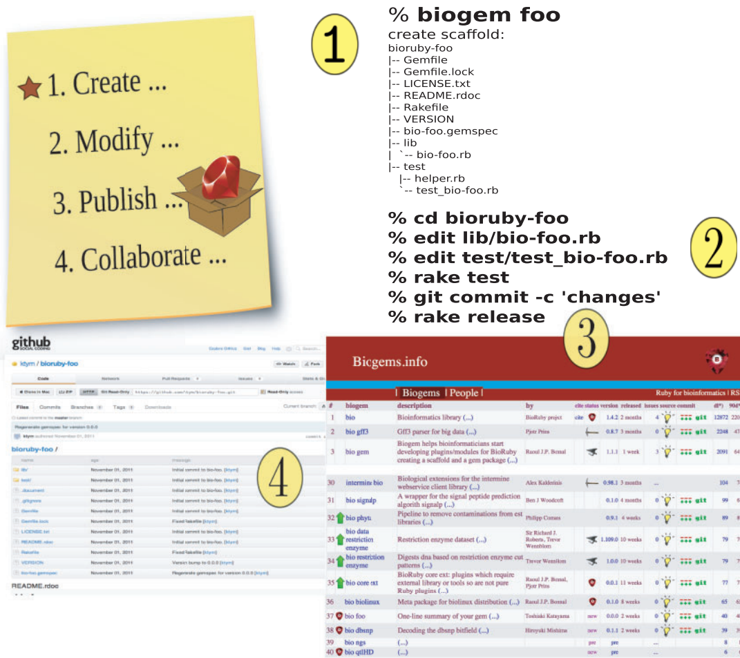
Fig. 1. Biogem eases publication of new bioinformatics Ruby software modules on the Internet, in a few steps. (1) The software generator creates the directory layout and files for a new software module named 'foo'. (2) The developer writes or modifies source code and (3) quickly and easily publishes the source code and module online, for others to read, install and use. Collaboration (4) is facilitated by publishing source code and changes to navigable websites. Then the workflow continues again at (2). The http://biogems.info website tracks published modules. Popularity of each published module is tracked, as well as source code changes, updates, bugs and issues. Unlike with the practise of publishing scientific papers, collaboration on software often comes post factum , i.e. after original publishing of a software module. Therefore, it pays to publish software modules early and often. This is reflected in the Biogem workflow.
