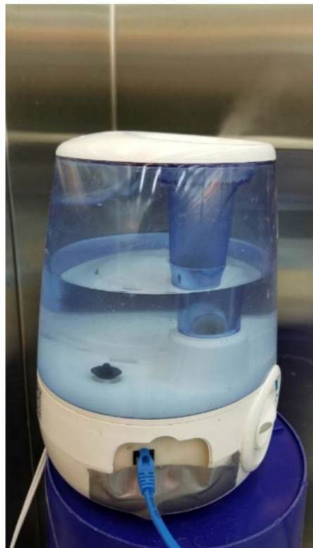
Figure 7. Assembled ammonia generator in operation.
