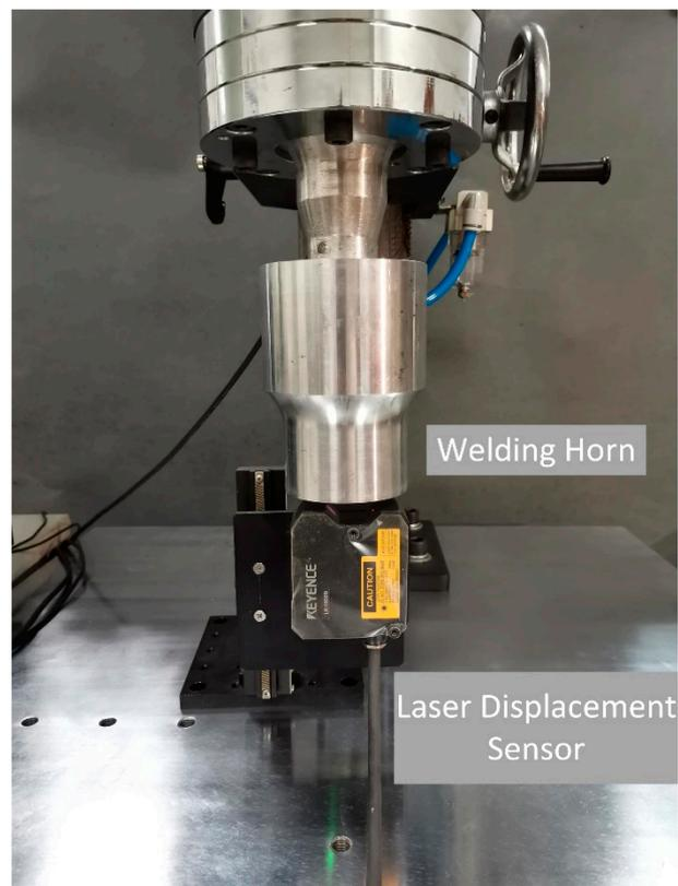
Figure 15. Experimental setup of vibration control verification.
