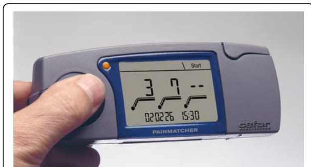
Figure 1 The PainMatcher instrument used for assessments of EST and EPT.
