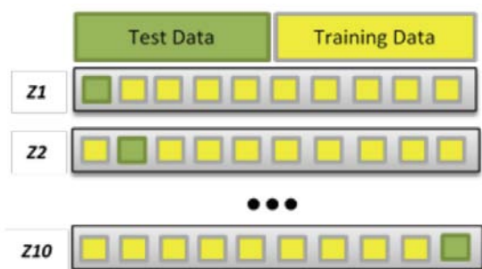
Fig. (8). Graphical illustration of 10-fold cross-validation. (A higher resolution / colour version of this figure is available in the electronic copy of the article).
