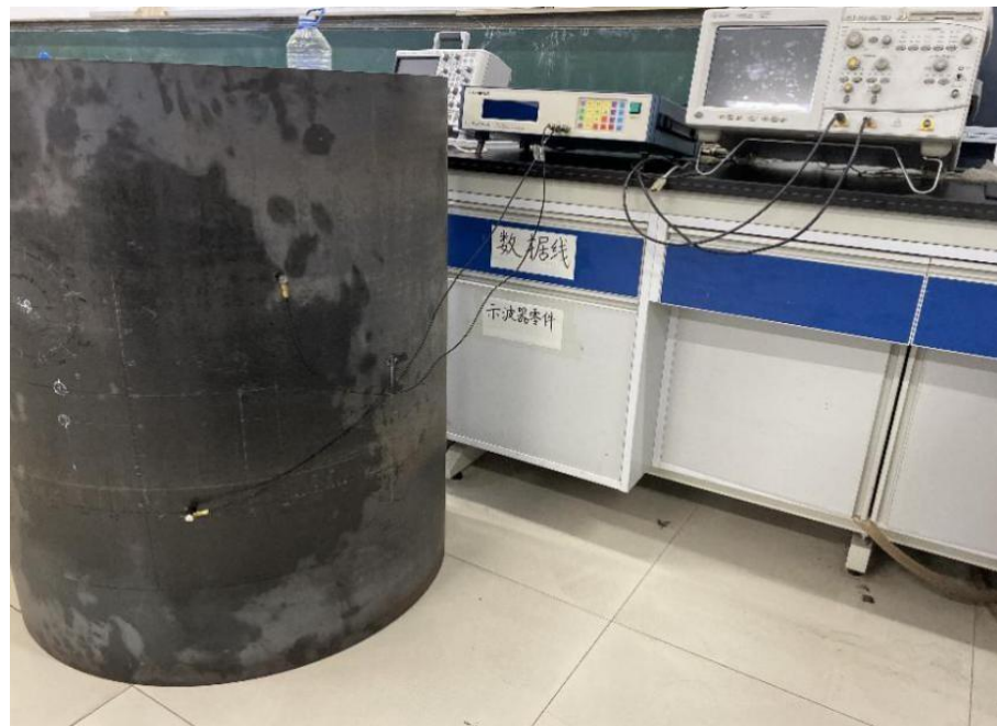
Figure 5. Experimental system. The experiment only uses two sensors to achieve acoustic source localization. One of the sensors is placed at the acoustic source position, and the second one at the receiver positions, marked before the experiment.
