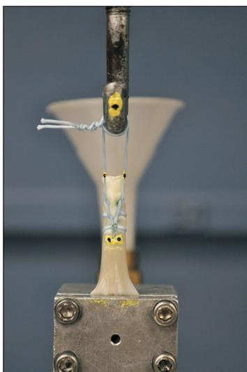
**Fig. 4.** Photograph of the suture-tendon construct mounted on the Instron material testing machine and knotted around the loading hook.
