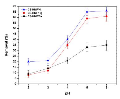
**Figure 2.** pH effect on the uptake of  $Ni^{2+}$ ,  $Hg^{2+}$ , and  $Ba^{2+}$ , from aqueous solutions (single-component) by using CS-HMF adsorbent.
