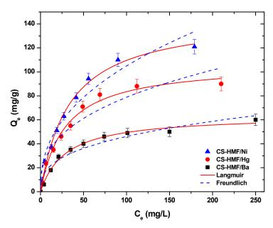
**Figure 5.** Equilibrium data for the uptake of Ni<sup>2+</sup>, Hg<sup>2+</sup>, and Ba<sup>2+</sup> from aqueous solutions (single component). Fitting to the equations of Langmuir and Freundlich. Testing conditions: T = 25 °C,  $C_0 = 10.0-300.0$  (mg/L), N = 160 rpm, V = 20.0 mL, t = 200 min, t = 0.02 g, pH = 6.
