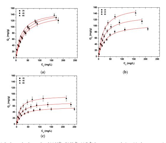
**Figure 6.** Isotherms for the uptake of (a) Ni<sup>2+</sup>; (b) Hg<sup>2+</sup>; (c) Ba<sup>2+</sup> from aqueous solutions (single component). Testing conditions: T = 25-65 °C,  $C_0 = 10.0-300.0$  (mg/L), N = 160 rpm, V = 20.0 mL, t = 200 min, m = 0.02 g, pH = 6.
