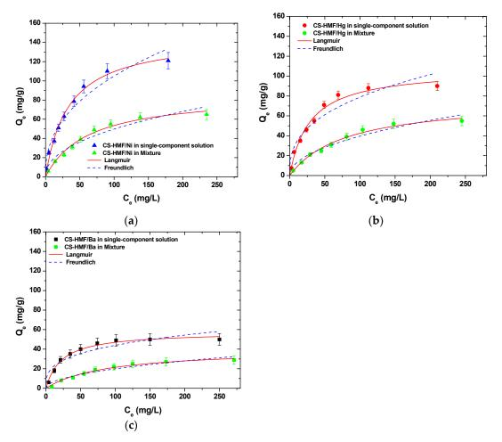
**Figure 8.** Equilibrium data for the uptake of (a)  $Ni^{2+}$ ; (b)  $Hg^{2+}$ ; (c)  $Ba^{2+}$  from single- and multi-component aqueous solutions, fitting to the equations of Langmuir and Freundlich. Testing conditions:  $T = 25 \, ^{\circ}C$ ,  $C_0 = 10.0–300.0 \, (mg/L)$ ,  $N = 160 \, \text{rpm}$ ,  $V = 20.0 \, \text{mL}$ ,  $t = 200 \, \text{min}$ ,  $m = 0.02 \, \text{g}$ , pH = 6.
