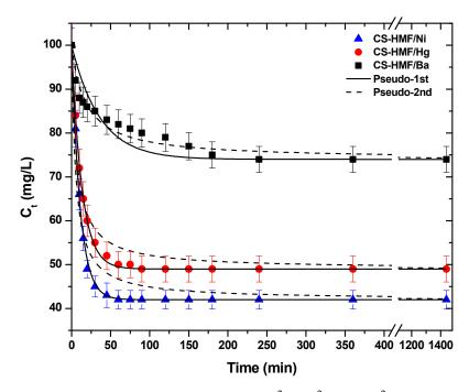
**Figure 4.** Kinetic data for the uptake of  $Ni^{2+}$ ,  $Hg^{2+}$ , and  $Ba^{2+}$  from aqueous solutions (single-component). Fitting to pseudo-1st and pseudo-2nd order equations. Experimental conditions: T = 25 °C,  $C_0 = 120.0$  mg/L, N = 160 rpm, V = 20 mL, m = 0.02 g, pH = 6.
