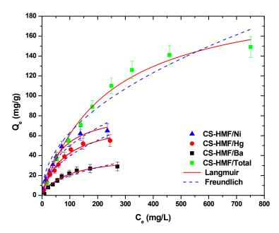
**Figure 7.** Equilibrium data for the uptake of Ni<sup>2+</sup>, Hg<sup>2+</sup>, and Ba<sup>2+</sup> in multi-component aqueous solution, fitting to the equations of Langmuir and Freundlich. Testing conditions: T = 25 °C,  $C_0 = 10.0–300.0$  (mg/L), N = 160 rpm, V = 20.0 mL, t = 200 min, t = 0.02 g, pH = 6.
