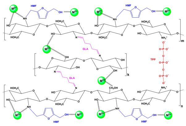
**Figure 3.** Proposed interactions for the removal of metal ions  $M^{2+}$  ( $Ni^{2+}$ ,  $Hg^{2+}$ ,  $Ba^{2+}$ ) by adsorption onto CS-HMF.
