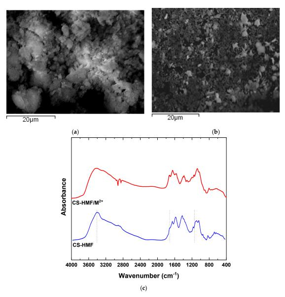
**Figure 1.** (a) SEM images of chitosan natural polymer 5-hydroxymethyl-furfural (CS-HMF) before metal ion removal; (b) SEM images of CS-HMF after metal ion removal (multi-component); (c) FTIR spectra of CS-HMF before and after metal ion removal.
