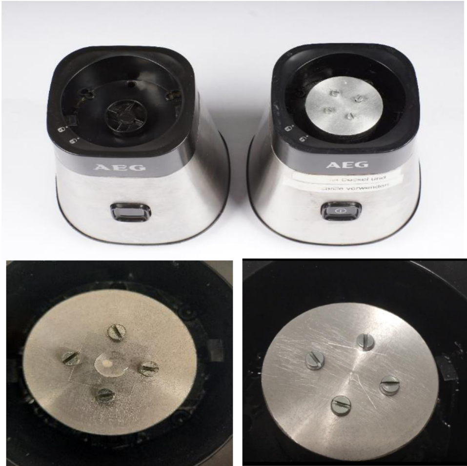
Fig. 2. Top: Smoothie maker before (left) and after the adaption for coverslip centrifugation; below: cover slip with honey drop and PEG before (left) and after (right) centrifugation
