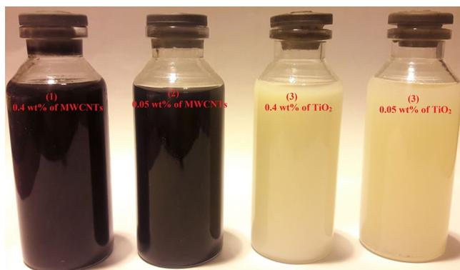
**Figure 8.** Camera pictures of nano lubricants after 2 h (1) 0.4 wt.% of MWCNTs, (2) 0.05 wt.% of MWCNTs, (3) 0.4 wt.% of TiO<sub>2</sub>, (4) 0.05 wt.% of TiO<sub>2</sub>.
