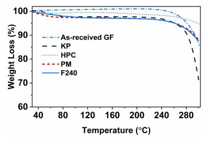
**Figure 5.** TGA thermograms of as-received GF, KP and HPC powders along with 3D printed tablet (F240).
