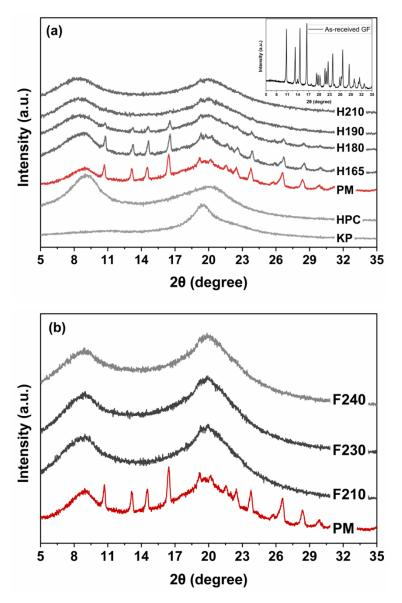
**Figure 3.** XRPD pattern of (**a**) as-received GF, physical mixture (PM), filaments through H165-210 and (**b**) 3D printed tablets, F210–F240.
