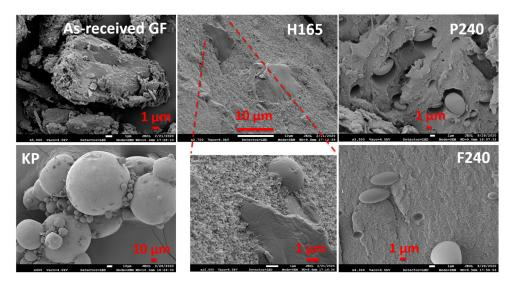
**Figure 4.** SEM images of as-received GF, KP powders, filament (H165), 3D printed tablet (F240) along with 3D printed placebo tablet (P240).
