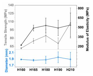
**Figure 1.** Mechanical properties and diameters of the filaments with varying HME processing temperatures, ranging 160–210  $^{\circ}$ C.
