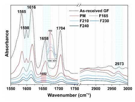
**Figure 2.** FT-IR spectra of as-received GF, physical mixture (PM) and 3D printed tablets through F165–F240.
