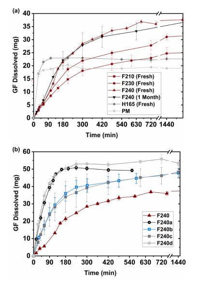
month at the ambient conditions, had comparable drug release performance to the freshly prepared F240, Figure 6a, indicating the presence of strong drug–polymer interactions.
