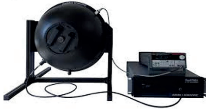
Figure 2. The radiant emittance values were recorded via spectrophotometric methods. (A) A laboratory-grade thermopile system. (B) A laboratory-grade integrating sphere spectrophotometer. (C) An in-office checkMARC portable spectrophotometer.
