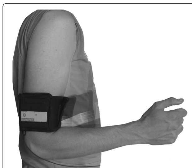
Figure 1 Fixation of Minimod device on upper arm with neoprene strap.
