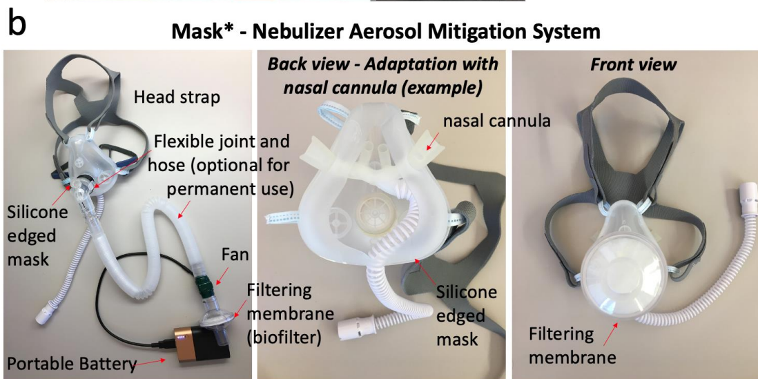
Figure 3. Different cases of combination of oxygen therapy and mitigation systems for nebulization. a) See text for description of Cases I-V. b) Silicone Mask* built for nebulization aerosol mitigation (see text for more details).
