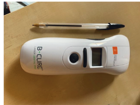
FIGURE 2: The device used for the treatment of the case, B-Cure Laser Pro (Erika Carmel, Haifa, Israel), emitting in the infrared spectrum (808 nm).
