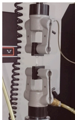
Figure 3. Specimen clamping during tensile test by Universal Instron Testing Machine 5500R.
