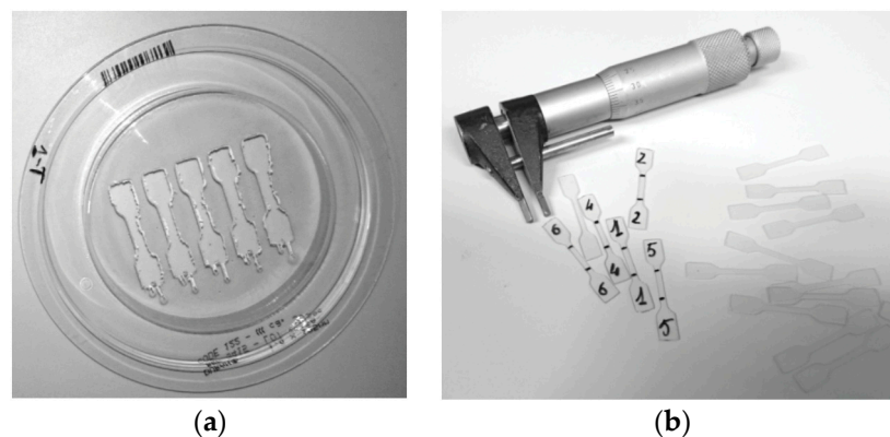
Figure 1. Thermoformed material after waterjet cutting (a) and resulting specimens (b).
