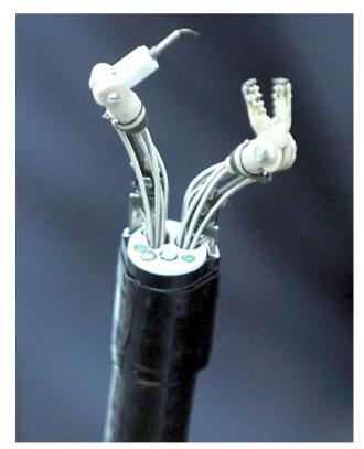
Fig. 3. The slave manipulator of the master and slave transluminal endoscopic robot (MASTER) system.
