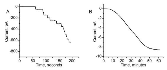
**Figure 1.** Lysenin channels reconstitution in artificial lipid membranes. (**A**) Shortly after lysenin addition, the ionic currents presented a discrete, step-wise, and uniform variation, indicative of individual channel insertion. (**B**) The macroscopic current reached a steady-state in  $\sim$ 1 h, indicative of insertion completion. Each plot represents a typical trace representative for the given experimental conditions.
